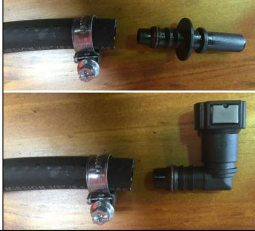
5. Disconnect the pick up line (the elbow clip) from the standard filter.
